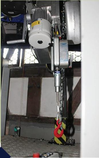
View of the electric rope hoist used in rescue operations
